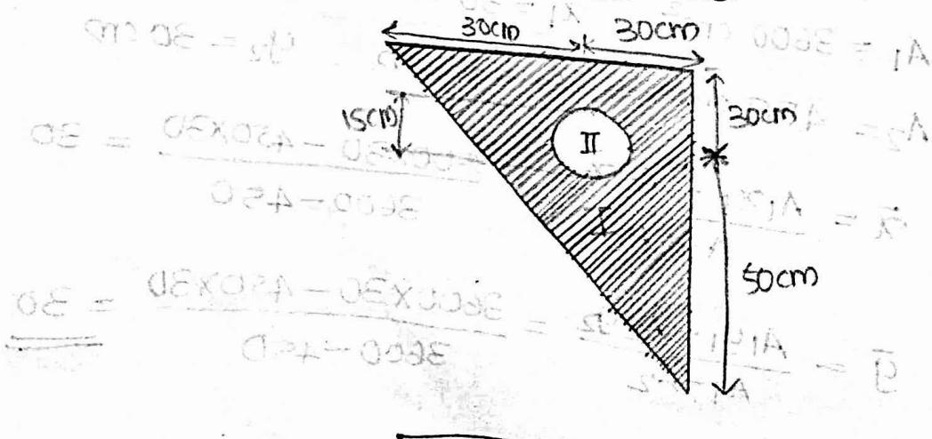
$$A_1 = \frac{1}{2} \times 60 \times 80 = 2400 \text{ cm}^2 \quad x_1 = 40 \text{ cm} \quad y_1 = \frac{2 \times 80}{3} = 53.33 \text{ cm}$$
