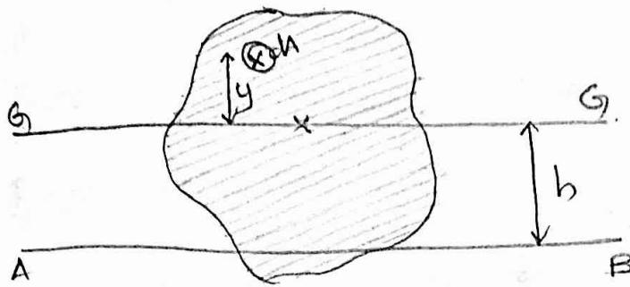
Consider an elemental area  $dA$  at a distance 'y' from centroidal axis. Then, moment of area about AB is  $(h+y)dA$  and second moment of area about AB is
