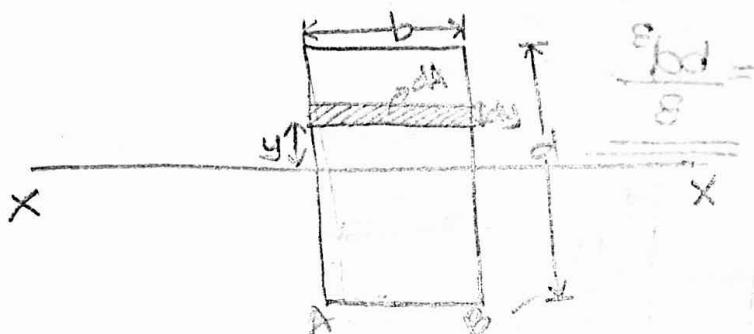
Consider a rectangular strip of thickness ' $dy$ ' at a distance ' $y$ ' from centroidal axis.
