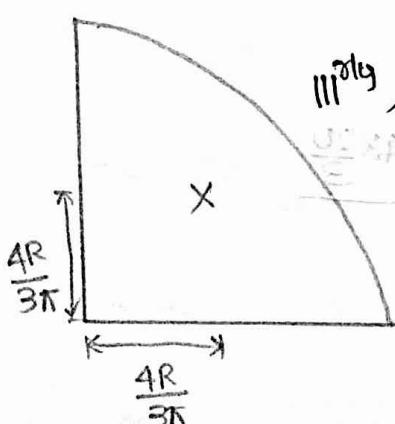
Thus, the distance of centroid of a semicircular lamina from its base is  $\frac{4R}{3\pi}$ .
